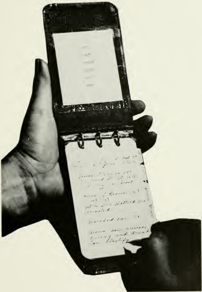
FIG. 2. Field Notebook, 3\frac{3}{4} by 6\frac{3}{4} inches. Note how this small, flexible book fits conveniently into the hand. This notebook can be used effectively under very adverse writing conditions.
